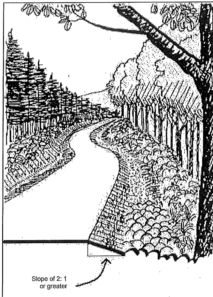
Roadside ditch draining to a rock diffuser set at least 50' from the water.
