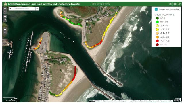
Figure A14. Example of dune crest elevation vs. 100-year FEMA Base Flood Elevation analysis from the <u>Coastal Structure and</u> <u>Dune Crest Inventory and Overtopping Potential Viewer</u>. Yellow and red circles indicate dune crest elevations below the 100-year BFE.
